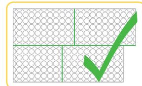
Recouvrement  $\geq 200$  mm
